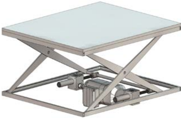
Scherenhubanlage / Scissor-lift system
